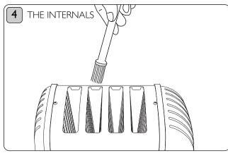
With the toaster unplugged use a **SOFT BRUSH** to clean inside your toaster, do not use a sharp or metal utensil! Crumbs should be carefully brushed off the elements using only a soft brush, the toaster can be turned upside down and excess crumbs be shaken out.
